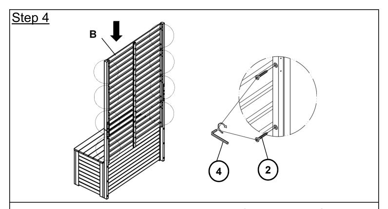
Attach the Back Panel(B) to Support Bars using Screws((2)) with Allen Key((4)) as pictured above.
