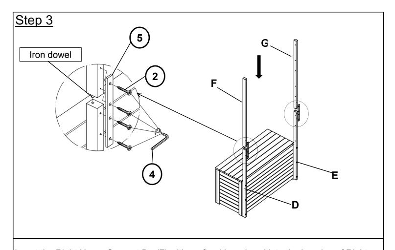
Insert the Right Upper Support Bar(F) with prefixed iron dowel into the housing of Right Lower Support Bar(D) as pictured above.
