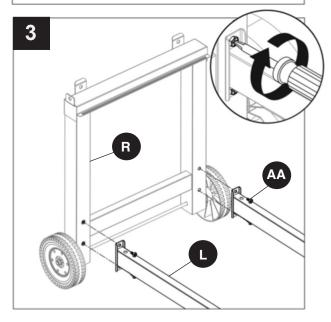
4. Attach two cart braces (L) to right leg assembly (M) using two M6x12 bolts (AA) on each side.
