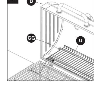
23. Fully tighten M6x30 bolts (GG) on each side of lid and firebox assembly (B).
