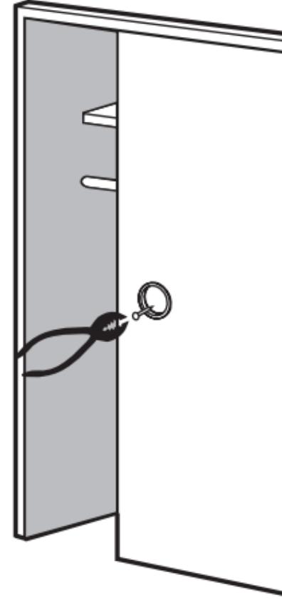
If nailed, pry out nails first on the edge of pull with a small screwdriver. Place new pull into hole and offset nail holes slightly from prior location to allow for a secure replacement.
