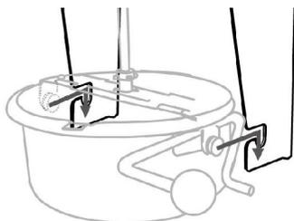
Assemble the kettle (B) on the supporters which are built into the main unit (A), and connect the cord from the unit to the socket in the ceiling.
