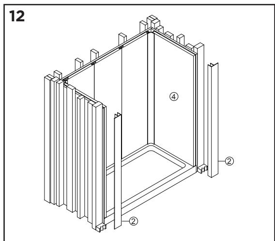
**IMPORTANT:** Properly caulk around the JETCOAT™ Shower Wall System to ensure a secure fit and finish. This includes, but not limited too:
