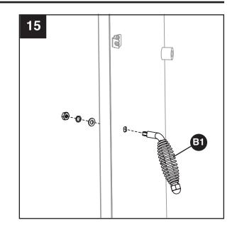
16. Attach the temperature gauge (B) by inserting the probe through the threaded opening on the smoker body door and turning clockwise.
