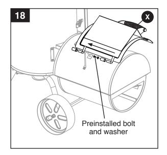
19. Install the side access door (D) onto the smoker body (A).
