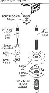
Use the MILWAUKEE FORCELOGIC™ Use the MILWAUKEE EXACT™ Adapter (Cat. No. 49-16-2685) with the Adapter (Cat. No. 49-16-2684) with M18™ FORCELOGIC™ 10T Knockout MILWAUKEE EXACT™ 2-1/2" to 4" Tool to properly fit other major brands of Dies on other major brands of tools with
