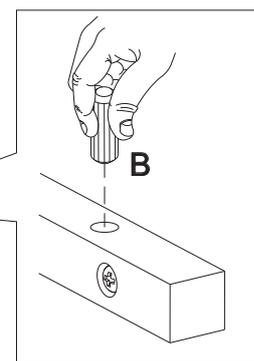
Insert wood dowel (B) into the front hole in the drawer rail (9).
