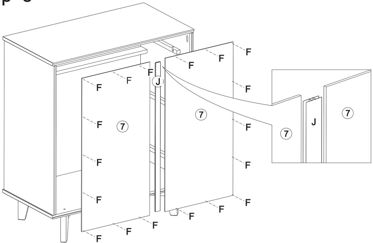
Secure back panel (7) with part (J) to body with nails (F)
