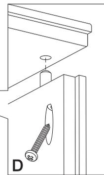
Use screw (D) to attach part (1) to body
