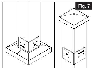
**Option B.** Remove template from rail kit. Align template with the base trim and post. Secure template in place using a piece of tape. Pre-drill through the desired marked locations on the template using a  $\frac{1}{8}$ " drill bit.
