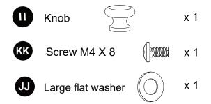
Note: Put screw (KK) through large flat washer (JJ) then through the end link of the retainer chain. Insert screw into hole on front door panel and attach the knob (II)
