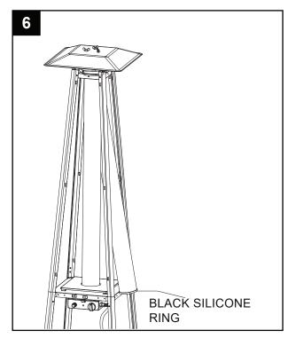
7.Assembly the protective guard (E). Hang the hooks of the protective guard (E) onto the holes in upper supports Secure the protective guards (E) with fixing brackets (GG) with 4pcs Screw 3/16" (HH).
