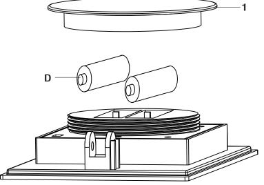
1. Twist off the battery cover, remove the old batteries and clean the battery contacts on the new batteries and solar lights. Replace with new 18500 Lithium 1000mAh rechargeable batteries and replace the battery cover (1).
