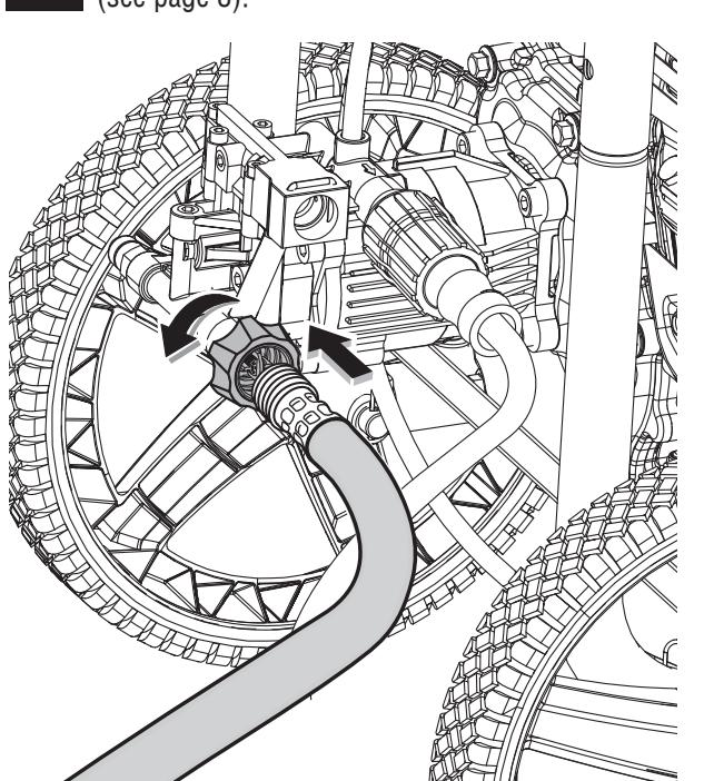
Completely uncoil garden hose or remove completely from reel to prevent kinks.
