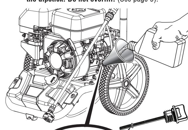
Turn the fuel valve to OFF before adding lubricant.
