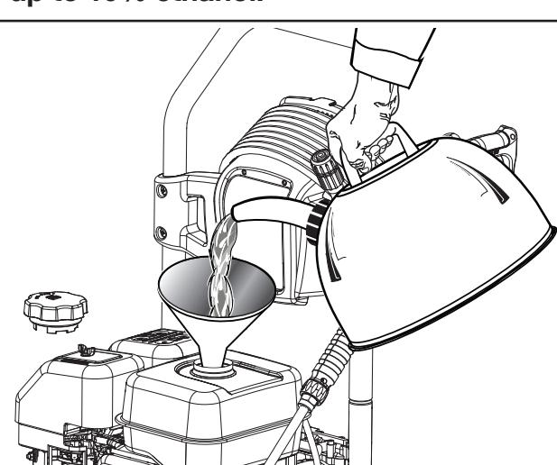
This is a 4-cycle engine. Do not mix fuel and lubricant together.
