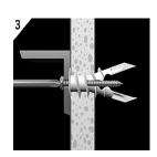
If you HIT STUD in drywall, do NOT use plastic anchors - Secure Screws Directly to Stud
