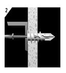
3. Tighten screw until flush with item.
