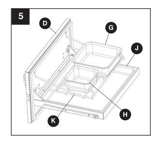
6. Slide the lower door assembly (D) onto the cabinet support rails as shown.
