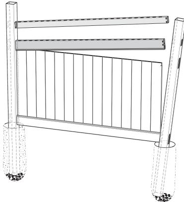
Insert the completed fence panel into the route holes of the second fence post. Plumb and level the post and add concrete according to manufacturers instructions.
