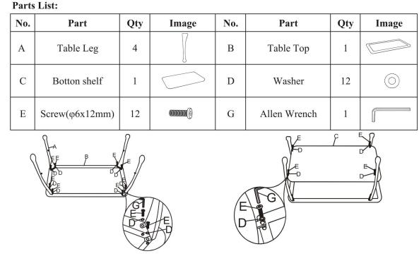
Step 1: Assemble 4 legs (A) with 8 washer (D) and 8 screws (E) by using allen wrench (G). Do not fully tighen now.
