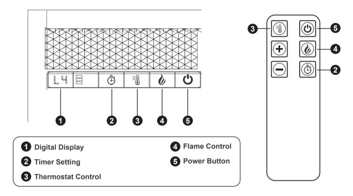
The buttons on the control panel and the remote control function in the same way.
