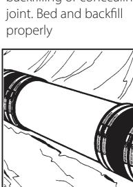
Tighten clamps to 60 in/lb. of torque. Pressure test before backfilling or concealing joint. Bed and
