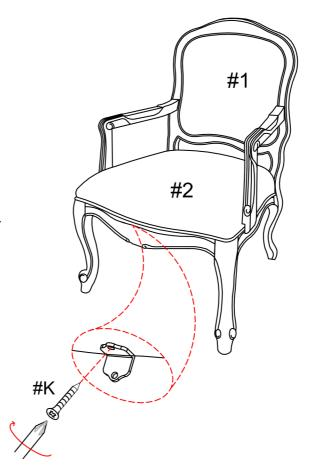
Carefully turn the completed chair upright. Make sure the chair is rested on a flat surface and does not feel loose or wobbly. If it does, double check that the bolts are secured and properly tightened.
