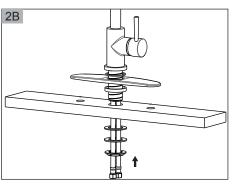
Install with deck plate. Position deck plate onto sink. Make sure the O-RING is placed at the bottom of the faucet base. Install faucet through hole in deck plate. From underside of sink, attach mounting assembly. Position faucet on deck plate properly and tighten Mounting Nut.
