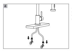
Open the water supply valve and flush for about a minute to clear the rubbish left in the pipeline, then turn off the water supply valve, and connect hot and cold water lines of the faucet to the water supply valves.
