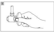
Remove any debris from valve outlets. Turning off the water supply valves.
