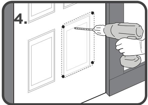
Drill a hole in all four corners with a minimum of 10mm drill bit.
