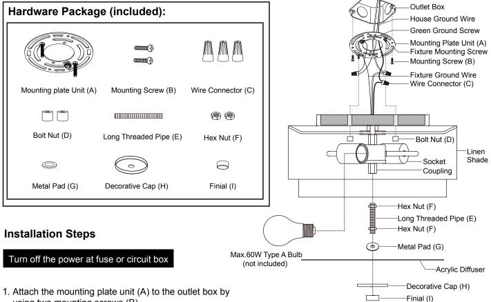
using two mounting screws (B).
