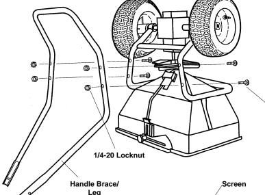
2. Attach leg/brace to frame as shown using (4) 1/4-20 x 2 1/2" carriage bolts and locknuts.
