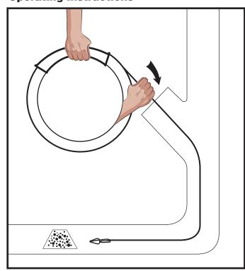
Extend the steel cable with boring head and feed into sewer drain.
