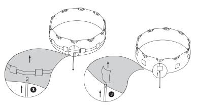
13. Go around and check that all fittings, legs, and beams are properly installed and secured in place. Make sure the drain fitting is plugged securely and the cap is in place.
