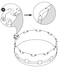
11. Carefully slide the Vertical Legs (3) up through the belt that runs around the middle of the pool.
