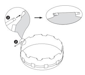
10. Insert the Pins down through the top of the T-Fittings until the Pins snap into place on the lower side of the T-fitting.
