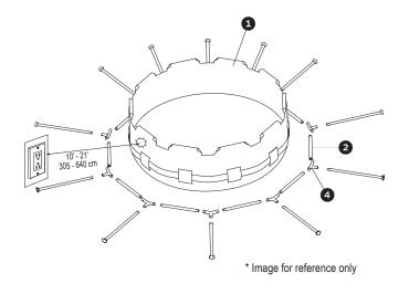
8. Carefully slide the Horizontal Beams **2** into the sleeves of the pool.
