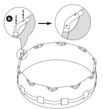
12. Look through the hole in the T-fitting, as you insert the Vertical Leg rotate it until the buttons align with the holes and pop out, locking the Vertical Leg in place. Do this for all Vertical Legs.
