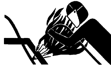
Heating Near Pressurized Fluid Lines
