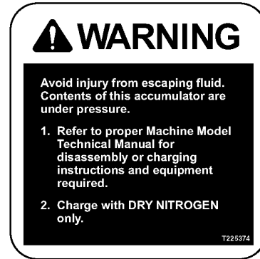
WARNING, Avoid Injury From Escaping Fluid
