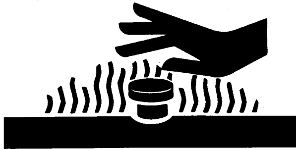
Surge Tank Warning
