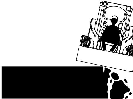
Operate on Solid Footing
