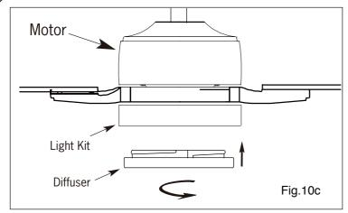
Install the guard to the light kit by the tightening 2 screws and washers. Screw the diffuser to the light kit.
