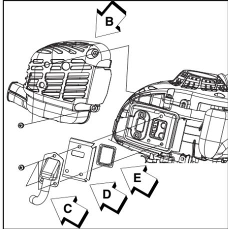
6. Replace screen if it is cracked, plugged, or has holes burned through.
