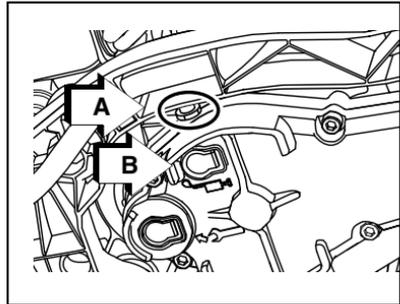
3. Remove the grommet next to the grease icon then add grease as illustrated.
