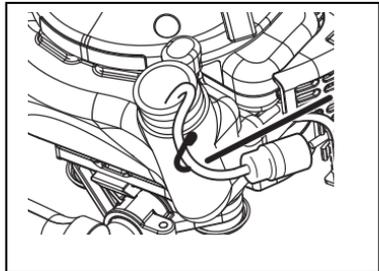
Note: Federal EPA regulations require all model year 2012 and later gasoline powered engines produced for sale in the United States to be equipped with a special low permeation fuel supply hose between the carburetor and fuel tank. When servicing model year 2012 and later equipment, only fuel supply hoses certified by EPA can be used to replace the original equipment supply hose. Fines up to \$37,500 may be enforced for using an un-certified replacement part.
