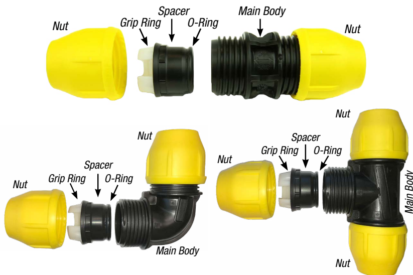
Figure 4.1 Fitting Re-assembly Diagrams
