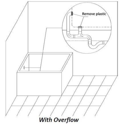
5.) Test the drainage to ensure that the water drains freely.
