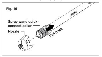
To disconnect a nozzle from the spray wand once the cleaning iob is complete:
