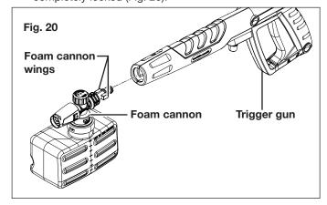
**5.** Turn on the pressure washer. Pull the trigger to operate the unit. The liquid detergent will automatically mix with water and be discharged through the nozzle.
