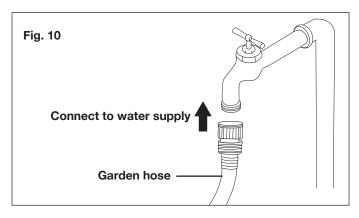
**WARNING!** Do not connect to potable water system.
