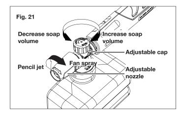
**WARNING!** Do not adjust the foam cannon while the trigger is squeezed. Failure to do so could result in damage.
