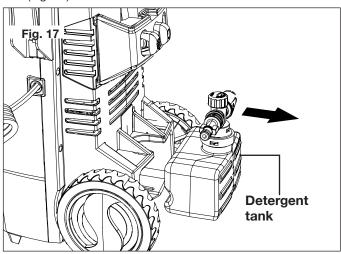
2. Remove the cap. Fill the tank or mix as recommended by detergent instructions (Fig. 18), and replace it back on the unit. Secure the cap back into place.
