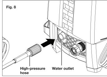
**WARNING!** Keep hose away from sharp objects. Bursting hoses may cause injury. Examine hoses regularly and replace if damaged. Do not attempt to mend a damaged hose.
