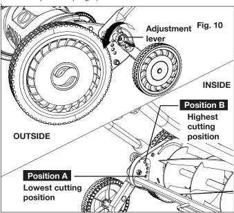
**4.** Other cutting heights are achieved by moving the adjustment levers to the settings between the highest and lowest positions.
