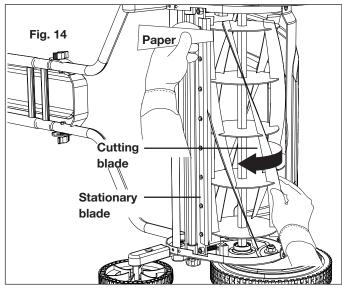
9. If most of the blades cut on both ends, the cutting system is set correctly. If all or most of the blades do not cut on one or both ends, the cutting system needs to be adjusted. Follow the instructions for adjusting the blade below.
