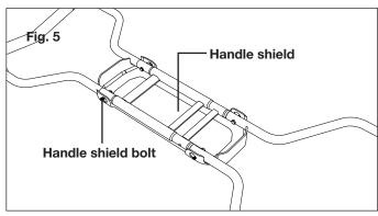
3. Align the handle shield knob with the bolt, then use your hand to tight. Repeat for the remaining three bolts (Fig. 6).
