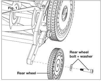
2. Use the supplied Allen wrench to secure the bolt (Fig. 2).
