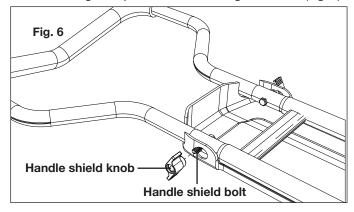
NOTE: Make sure all the bolts and knobs are secured.
