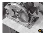
**Cut panels to accommodate shower heads and faucets.** Measure and mark the borders where the opening will be with a marker. Drill a 1/2-inch to 1-inch hole using a drill in a corner of the cut-out section (image 9). Use a jigsaw or hole saw to cut the remaining opening, following your tracing (image 10, 11).
