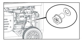
6c. When gasoline stops flowing from the carburetor, replace and tighten the carburetor drain bolt and be sure to properly dispose of the drained gasoline according to local regulations or guidelines.
