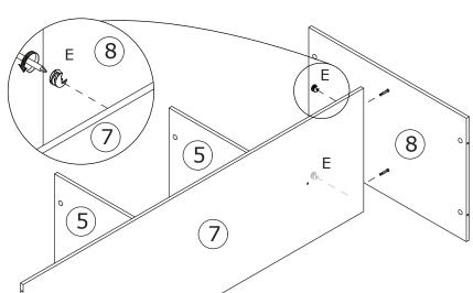
Attach board 8 to board 7, put cam lock(E) into holes in board 7 and turn clockwise to tighten as shown.
