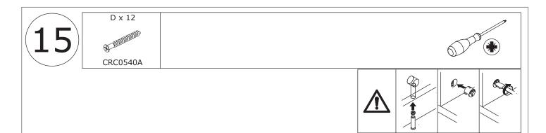
Then fix plate 4 to plate 11,7,6 and 1 using screw(D) as shown.
