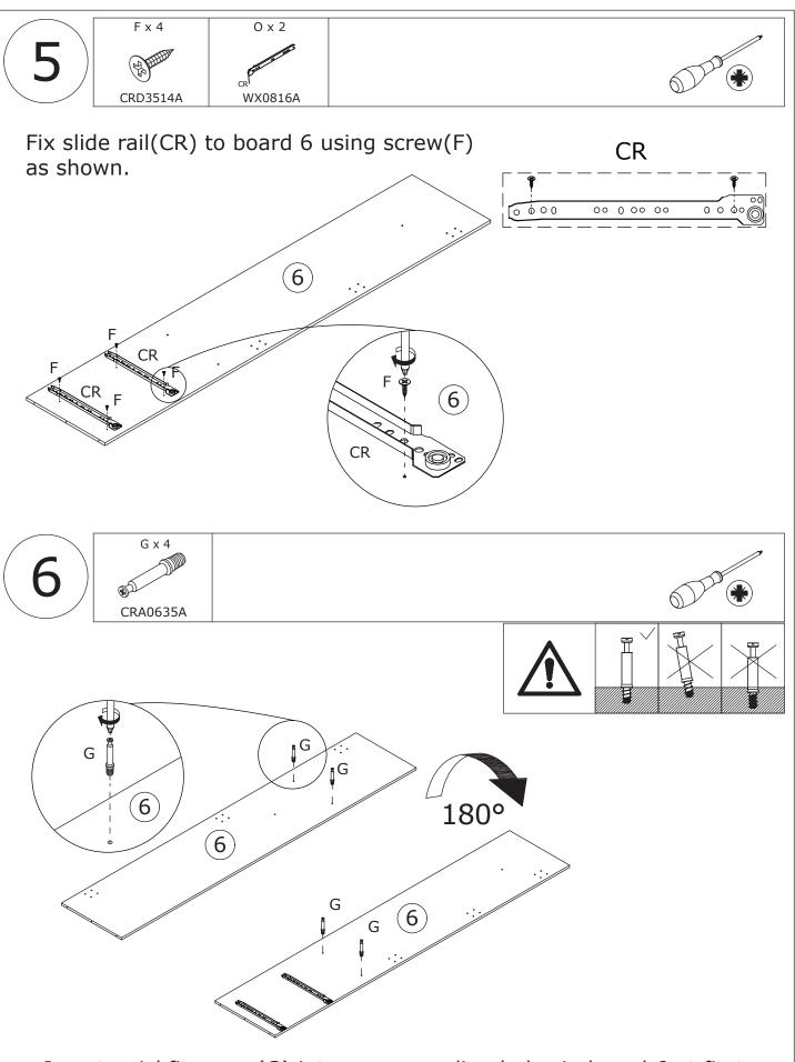
Insert quickfit screw(G) into corresponding holes in board 6 at first. Flip the plate, insert quickfit screw(G) as shown.
