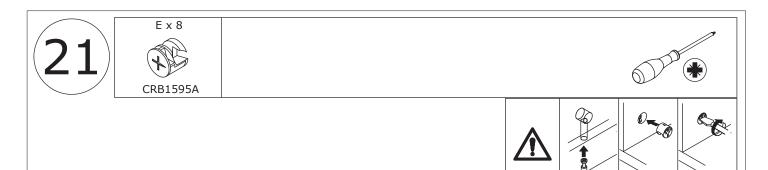
Attach the frame to board 4, put cam lock(E) into holes in board 2,16 and turn clockwise to tighten as shown.
