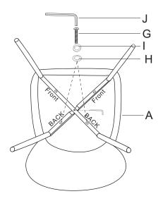
STEP 3: Use bolt G, spring washer I, flat washer H to connect rear holes of legs with bottom of the seat. Make sure all holes on legs align with holes on bottom of seat then fasten all bolts to secure.
