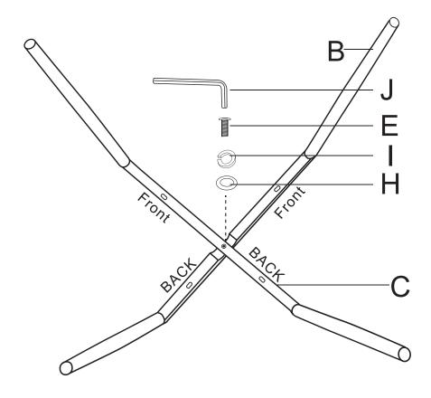
STEP 1: Use bolt E, spring washer I, flat washer H, allen wrench J to connect metal leg part B and C together, don't fasten the bolt at this stage.
