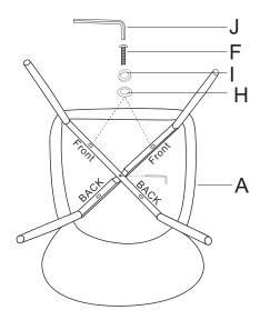
STEP:2 Use bolt F, spring washer I, flat washer H, allen wrench J to attach the Front part of the legs assembly to bottom of the seat.
