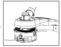
Trimmer head is now fully loaded and ready for operation.
