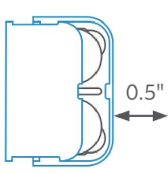
Leave at least a 1/2 inch (12.7 mm) space so you can open the battery compartment.
