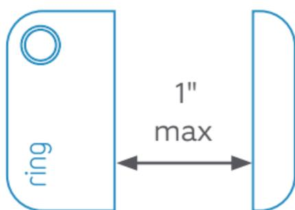
Ensure no more than 1 inch (25.4 mm) between sensor and magnet when the door or window is closed.
