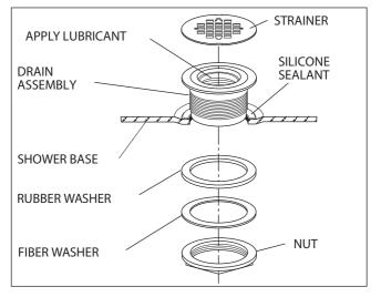
Remove the stainless steel strainer from the drain assembly. Disassemble the locknut and two gaskets from the back of the drain assembly. Apply a 1/4" bead of caulking (silicone) to the drain hole and insert the drain assembly. Replace the rubber washer, fiber washer, and lock nut in that order. Hand tighten the locknut. Remove excess sealant from finished side.
