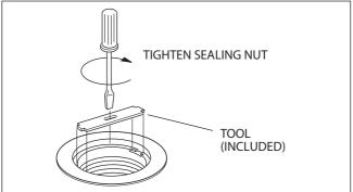
Remove the tool, locking mechanism and rubber seal from the inside of the shower drain. Lubricate the seal with common household liquid soap and slide it over the 2" drain pipe. With a large screwdriver and the tool provided, tighten the compression nut to seal the drain pipe connection. After the drain is fully installed check for proper drainage and inspect for leaks.
