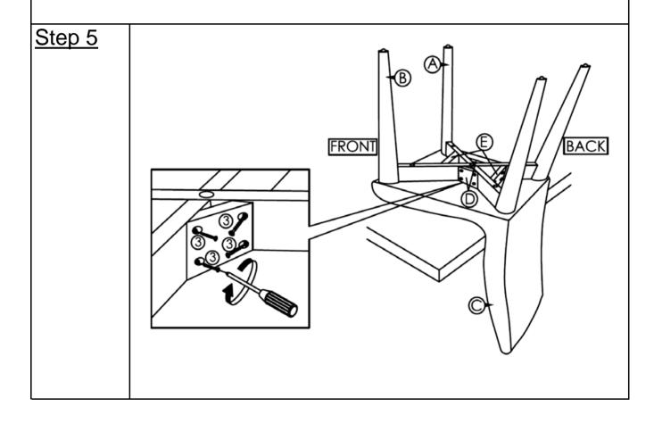
Place the Corner Blocks(D) at the side joints of Leg(A) and Leg(B) as shown. Place the Corner Blocks(E) at the front and back joints of Leg(A) and Leg(B) as shown.
