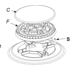
The ignitor must be cleaned very carefully.
