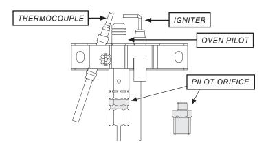
In the pilot assembly shown below, the LPG orifice is 0.14 mm. When doing the conversion from Propane to Natural gas make sure the pilot orifice is changed to the NG orifice sized at 0.2 mm. If you leave the LPG orifice 0.14mm in place, the pilot flame will may be too small to keep the pilot lit.
