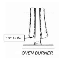
Oven burner flame can be checked as follows (without flame spreader in place):
