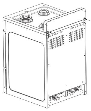
2. Secure the backsplash to the cooktop from the back using the 2 Phillips head screws provided as shown in the diagram.
