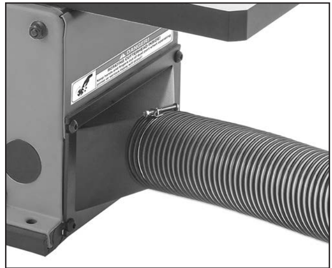
Figure 17. Dust hose attached to dust port.
