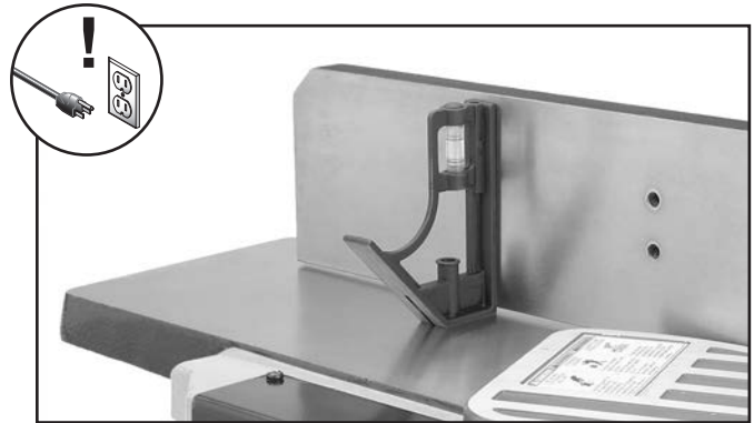
Figure 54. Example of checking 90° fence angle with combination square.
