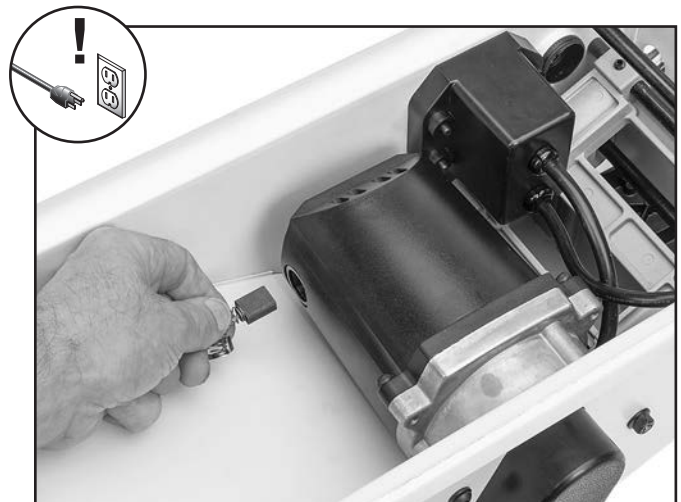
Figure 60. Example of removing motor brush.
