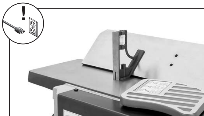
Figure 56. Example of checking 45° fence angle with combination square.
