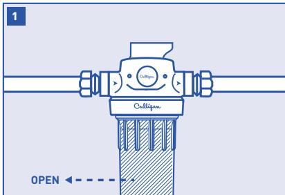
Turn water off by rotating bypass valve to "Off" or "Bypass."
