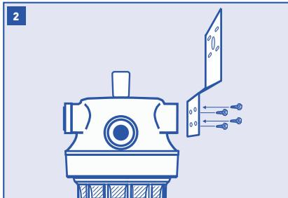
If using optional BR-C mounting bracket, start by making sure the arrows facing you on the system are consistent with the direction of your water flow. If necessary, remove filter life indicator holder if on the back side of the unit, and move it to the front. Align the holes of the bracket with the holes on the back of the filter head. Insert four mounting screws through the bracket and into the filter head until tight. Otherwise skip to step 3.
