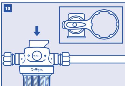
Ensure the filter housing has been properly tightened using the housing wrench provided.
