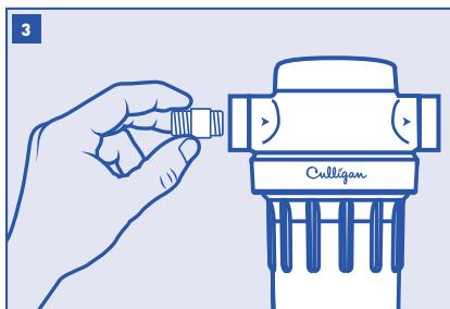
Assemble all fittings. Start adapters (not included) into filter head by hand. Use a wrench to tighten firmly.
