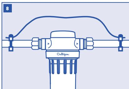
**CAUTION:** If water pipes are used to ground electrical systems, appliances or phones, be certain to install a jumper wire.
