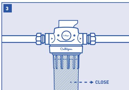
Screw the bottom of housing onto the cap until tight. **DO NOT OVER-TIGHTEN.** Make certain standpipe in filter head slips into cartridge.
