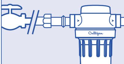
Align filter assembly with ends of pipe, making certain your water flow is in the same direction as the arrows on your filter head. It will be necessary to spread ends of pipe apart to install filter assembly. Using two adjustable wrenches, hold incoming fitting securely with one wrench and tighten nut with second wrench. Repeat process for outgoing fitting.
