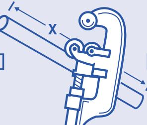
Using a pipe cutter or hacksaw, cut and remove marked section of pipe. File or sand sharp edges on remaining pipe.
