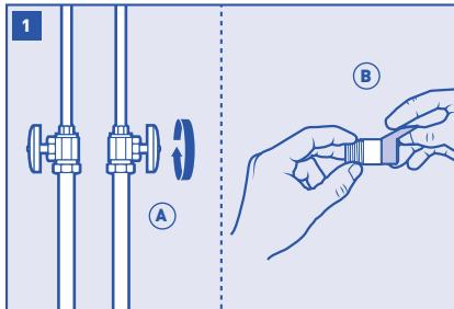
Turn off water supply (A) and open nearest faucet to drain pipes before installation.
