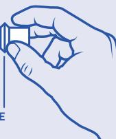
Slip brass compression nut and ferrule onto each end of 1" pipe.
