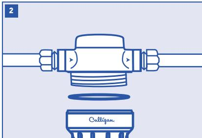
Lubricate O-Ring with a coating of clean food-grade silicone grease. Insert O-Ring back into groove and smooth into place with finger.
