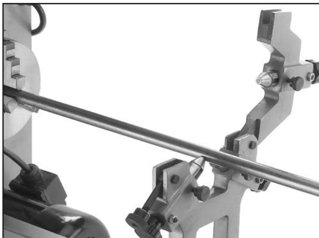
Figure 33. Loading the workpiece into the steady rest.
