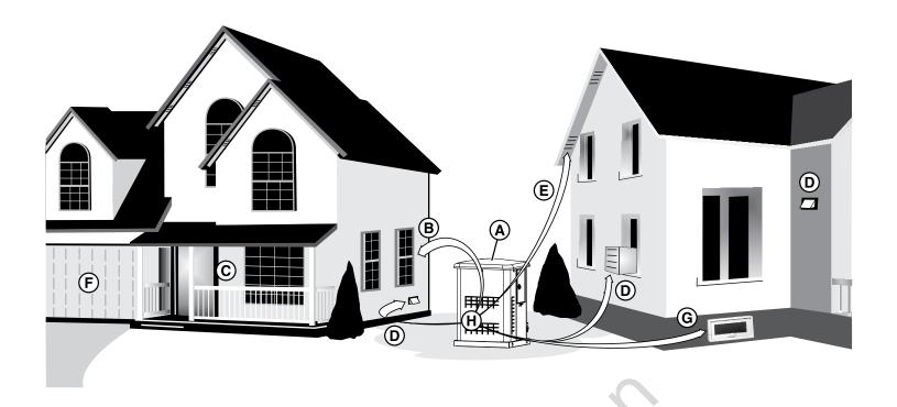
All fossil fuel burning equipment, such as standby generators (A), contains carbon monoxide (CO) gas in the engine exhaust. CO gas is odorless, colorless and tasteless and is unlikely to be noticed until a person is overcome. CO gas can kill you, so it is required that the following is included as part of the installation.
