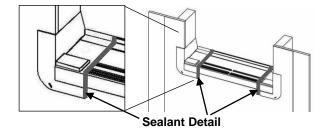
**E**. Fold SureSill™ FlexCap™ on back side to complete end dam. Repeat the same for other side.
