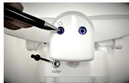
Push this latch switch under Sensor head by a finger, pen or screwdriver to "click" ON
