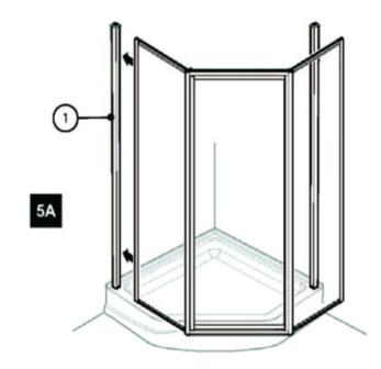
5B-5C. Engage the other side of assembly into wall jamb(#1)
