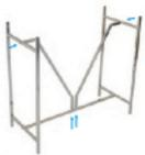
Attach another end of each V- bar to the central hole of support bar
