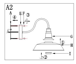
6.Attach mounting plate A to outlet box by mounting screw B (REFER TO CHART A3)
